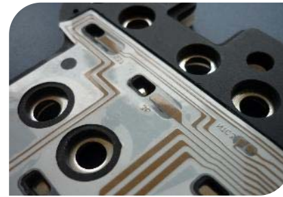
Interconnection Boards for Batteries
