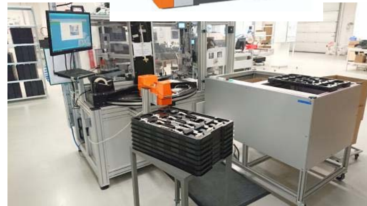
EOL functional test
